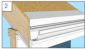
Bend the upper part of the flashing to the proper roof angle (or specify the angle and have us bend it for you).
