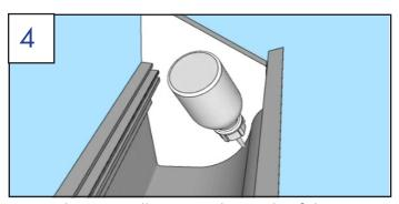
Apply 2P-10 Adhesive to the inside of the gutter next to the plug.
