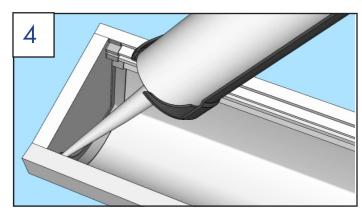
Apply sealant to inside of plug, including the grooves in gutter.
