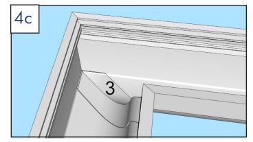
Install 3rd piece of tape on right side of joint.
