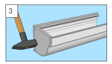
• Tap the plug flush with the end of the gutter.
