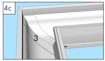
Install 3rd piece of tape on left side of joint.
