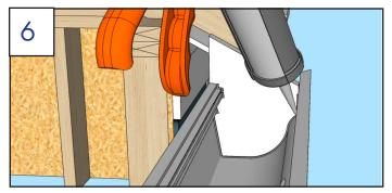
Apply sealant to the inside of the plug, including the grooves in gutter.
