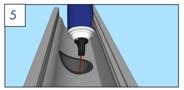
Spray perimeter of hole with 2P-10 Activator.
