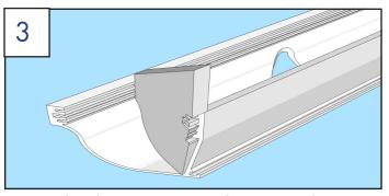
• Tap the plug part way into the gutter, taking care to align the edges.
