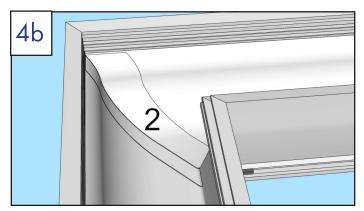
• Install 2nd piece of tape on right side of joint.
