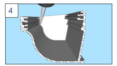
Apply sealant to the inside of end cap, including in grooves in gutter.
