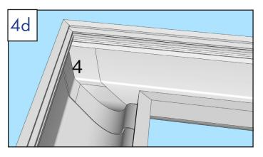
• Install 4th piece of tape on inside corner of joint, starting at the top.
