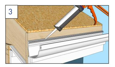
For extra protection against ice dams, apply sealant in the top groove before installing flashing.
