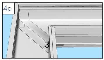
• Install 3rd piece of tape on back of joint.
