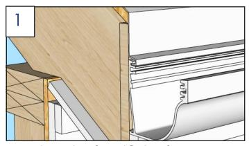
Pre-bent edge of metal flashing fits into top groove inside gutter. Flashing should be installed over waterproof roof membrane layer (not pictured), and then taped to seal joint between membrane and flashing.
