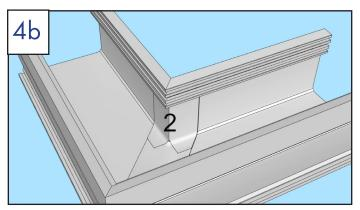
• Install 2nd piece of tape on front of joint.
