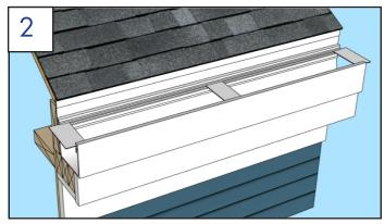
Install supplied leafguard supports at each end of leafguard, and in middle. See below image for correct grooves in gutter.
