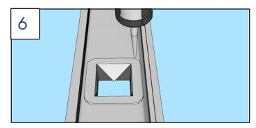
• Apply Dicor sealant over edges of tape.
