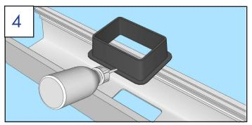
Apply 2P-10 Adhesive to bottom lip of outlet and insert outlet in gutter.
