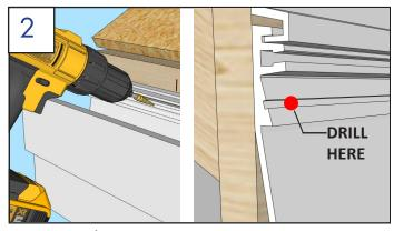
• Drill a 7/16" hole centered on the angled shelf inside gutter.
