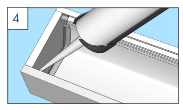
Apply sealant to inside of plug, including the grooves in gutter.
