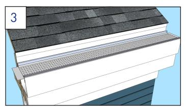
Install leafguard by pushing it into the back groove first, then snapping it into the front groove.
