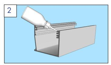
Apply 2P-10 Adhesive to edge of gutter.
