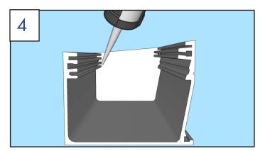
Apply sealant to the inside of end cap, including in grooves in gutter.
