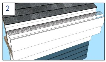
Bend the leafguard up slightly in the middle of the mesh, so it can fit inside the grooves in the gutter.
