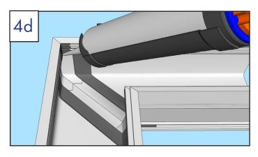
Apply sealant in the grooves above the tape, and over the sides of the tape.
