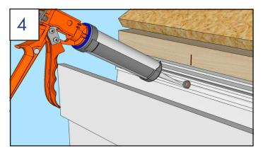
• Cover the screw head and washer with sealant.
