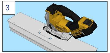
Cut between holes with jigsaw (cover jigsaw base with tape to avoid scratching gutter).
