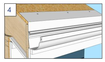
Install flashing in top groove inside gutter and nail to roof. Each piece of flashing should overlap adjacent pieces by 3".
