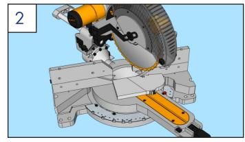
Remove plug and cut at roof pitch angle on miter saw.
