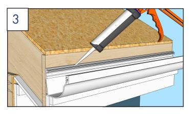
For extra protection against ice dams, apply sealant in the top groove before installing flashing.
