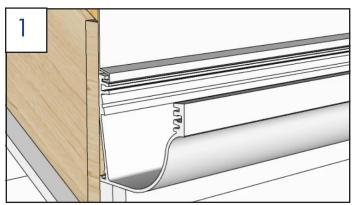
Pre-bent edge of metal flashing fits into top groove inside gutter. On membrane roof (e.g. EPDM), flashing should be installed after membrane, and cover tape should be installed over flashing. On shingle roof, flashing should be installed before Ice and Water Shield.
