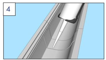
Apply sealant in the grooves above the tape, and over the sides of the tape.
