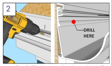
Drill a 7/16" hole centered on the angled shelf inside gutter.
