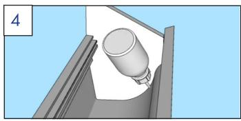
Apply 2P-10 Adhesive to the inside of the gutter next to the plug.
